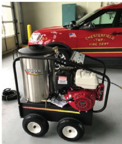
Heated high pressure washer for cleaning and decontamination.
